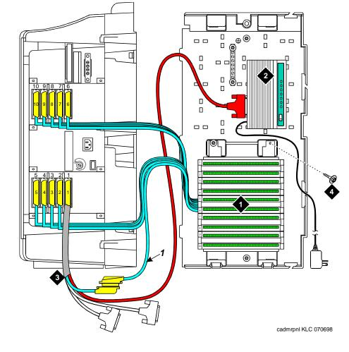
Figure 16: Typical Bottom-Mount MDF and Modem Cable Routing
